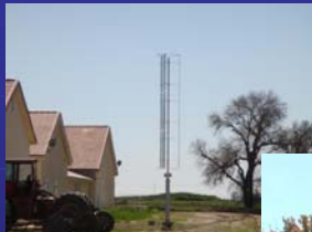
Windspire – Vertical Axis Turbine
