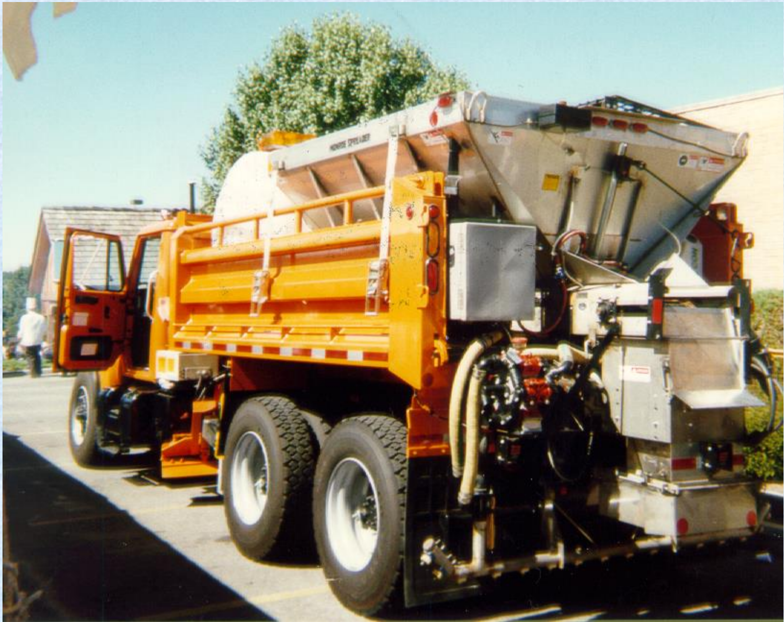
Pre-wetting ice control equipment
